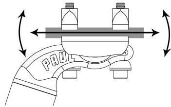
Once properly positioned, use a torque wrench to finish tightening the clamp screws to **90 in-lb** (10.1 Nm). Test ride and readjust if necessary.
