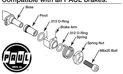
mounted on the correct side of the brake. Brake springs are directional and must be
