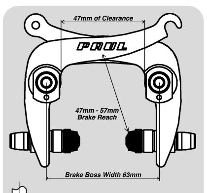
Brake Boss Height 700c = 340 mm 650b = 321 mm 26" = 309 mm The Braze On Racer Medium mounts directly to brake bosses on the frame and has greater stiffness and stopping power.
