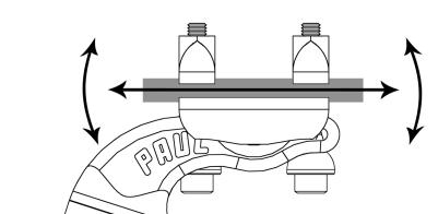
Once properly positioned, use a torque wrench to finish tightening the clamp screws to **90 in-lb** (10.1 Nm). Test ride and readjust if necessary.
