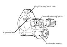
Read and familiarize yourself with the instructions for your dropper seat post. Clamp the Dropper Trigger to the handle bar with a torque recommended by your handle bar manufacturer.
