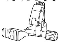
The PAUL Dropper Trigger can be used with most cable operated dropper seat posts. There are provisions for the cable head and a cable clamp if the head is used on the seat post.
